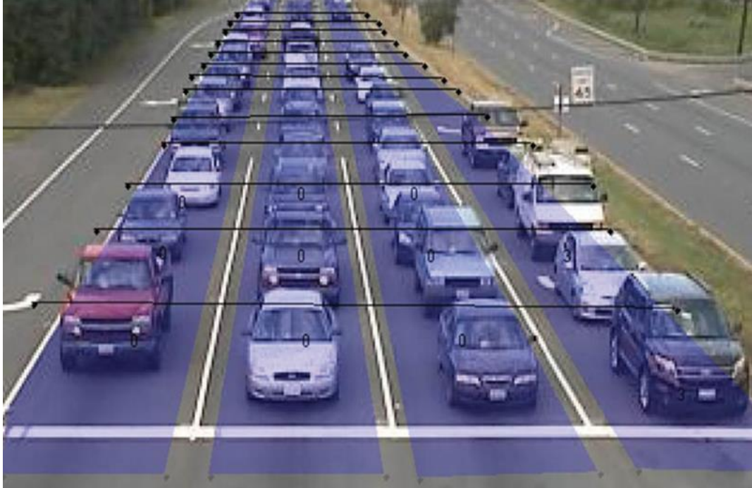
Figure 14. Vehicle counting concept of InSync based on cameras (Ta, 2016).
